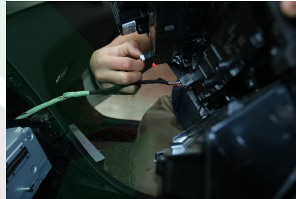
5. Plug the LVDS cables from the head unit
