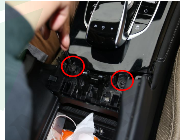
3. Remove the two screws
