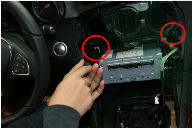
6. Remove the screws from head unit
