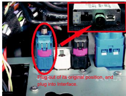
6. Unplug the OEM LVDS cable from the back of the head unit and connect it into the interface module as shown above.
