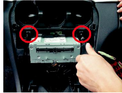
3. Remove the Command System from the center console to access the LVDS and Quadlock connections.
